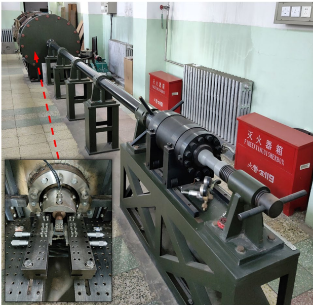
Fig. 3 The actual ultra-high-speed cutting experimental setup. The insert shows the cutting platform
