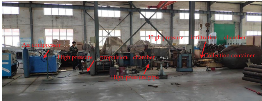
FIGURE 2: Platform for bauxite ore powder production.
