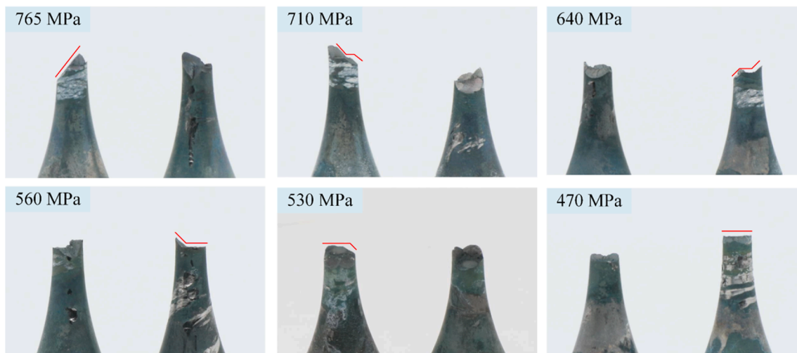
Fig. 6. The macro fracture morphology of specimens under different stress levels.
