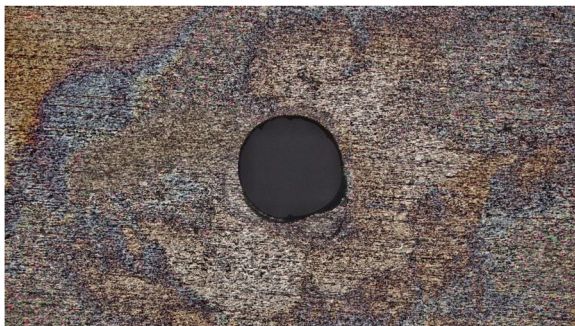
FIG. 19. Sputtering corrosion of the extractor caused by multipoint emission ( d_1 = 0.5 mm).
