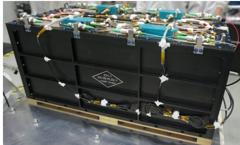
Fig. 2. The IECB of Taiji-1 interferometer assembled together with the modulated part of the interferometer which also contains AOMs and an optical fiber beam splitter.
