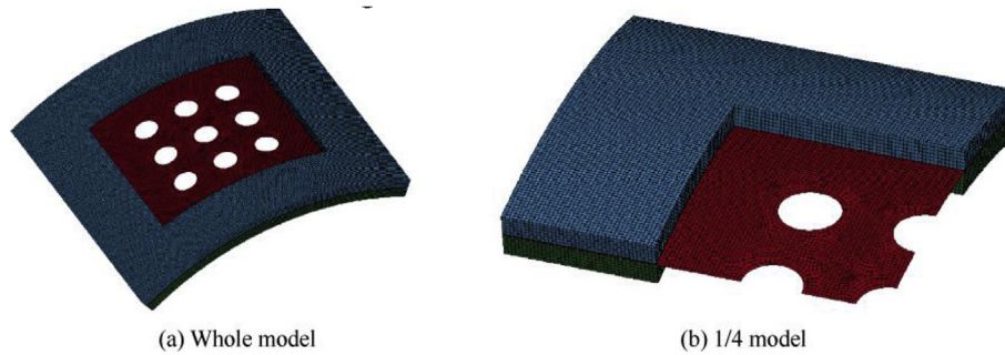
Fig. 10. Finite element model of cylindrical shell with pre-formed holes.
