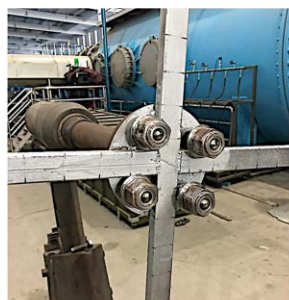
(b) 钢丝悬挂加载结构 (b) Steel wire suspension structure
