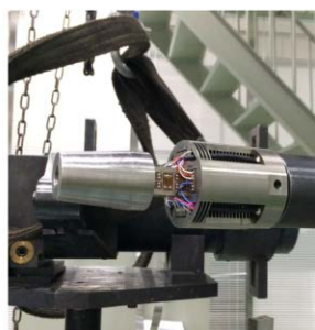
(c) 脉冲型应变天平 (c) Impulse strain gauge balance
