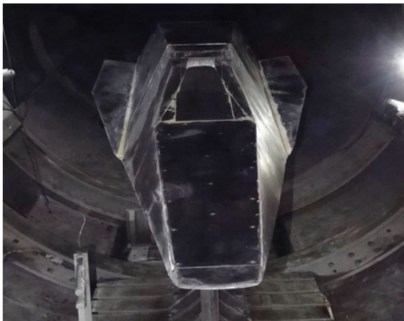
Fig. 6 Performance Test Engine mounted in the JF12 hypervelocity shock tunnel
