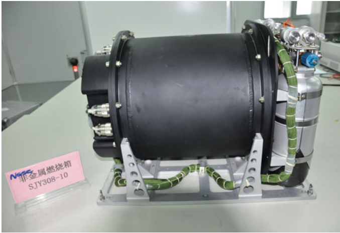
Fig. 10 Flight hardware of the microgravity experiment aboard the SJ-10 satellite
