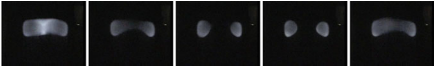
Fig. 13 Sequence of front-view images of flame oscillations during flamelets formation at an oxygen concentration of 40% after the flow speed is decreased from 6 to 3 cm/s. The images are separated by an equal time interval 0.08 s
