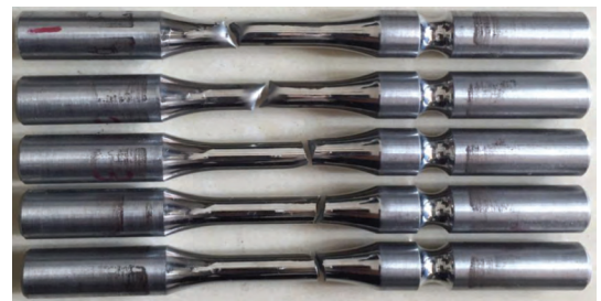
图 11 轴向应力疲劳沙漏+狗骨形试样疲劳破坏照片 Fig. 11 Pictures of failed hourglass + dogbone specimens under axial fatigue test
