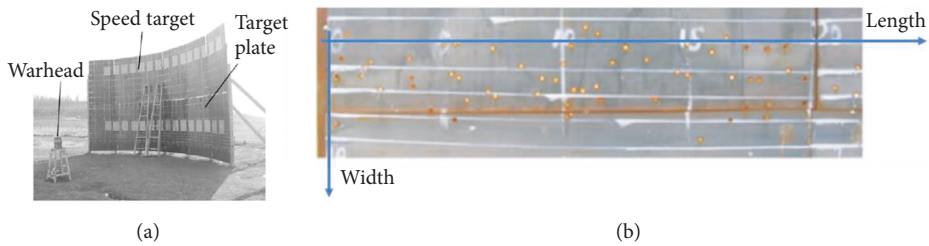
FIGURE 4: (a) Test site layout; (b) witness plate with some fragments.
