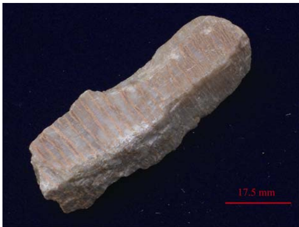
Fig. 1. An antiperthitic intergrowth of K-feldspar (the veinlets) in the Na-feldspar (this hand specimen has 7 cm length and 3 cm width from Eurico Zimbres in Wikimedia in 2006).
