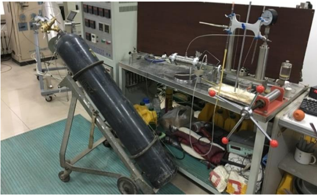
Fig. 4 The set-up diagram for stress-dependent permeability.
