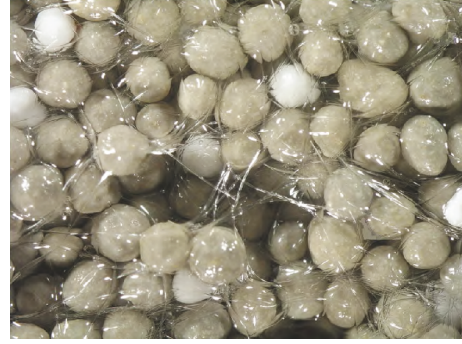
FIGURE 1: Network structure of fibers and proppant mixture [6, 7].
