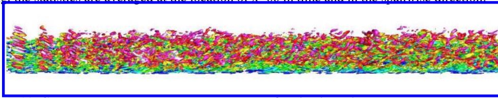
Figure 11. Coherent turbulent structures based on Q-criterion with mapped-on local Mach number
