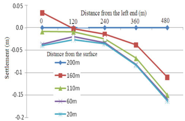
Figure 3. Changes of displacement vertical to slope surface at different depth. (This figure is available in colour online.)
