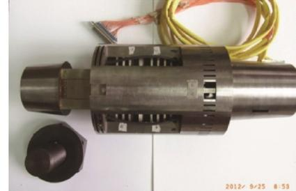
**Fig. 5** Six-component stress balance designed for JF12 shock tunnel.
