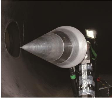
**Fig. 3** 10° half-angle cone model installed in JF12 shock tunnel.
