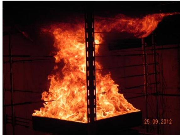
Fig. 4. Figure of flame impinging to the ceiling
