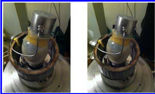
Figure 3. Specimen after experiments by depressurization.
