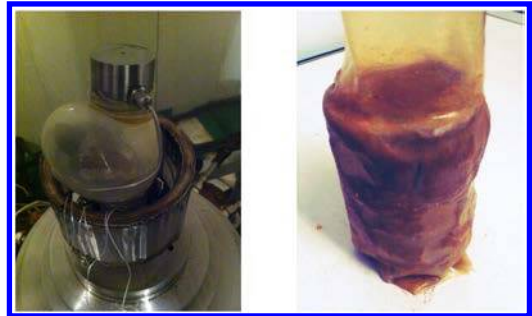
Figure 6. Specimen after experiments by thermal stimulation.
