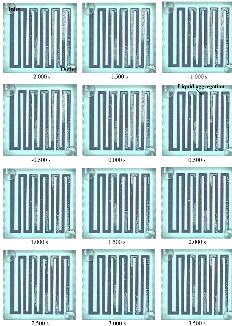
Fig. 10. Two-phase flow in the cathode flow channel under normal gravity/microgravity conditions at low current density.
