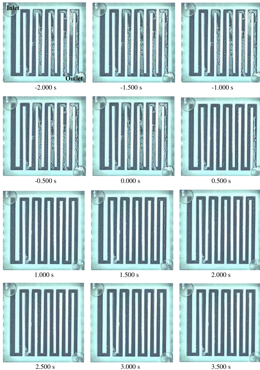
Fig. 7. Two-phase flow in the cathode flow channel under normal gravity/microgravity conditions at high current density.
