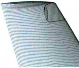
图8 WENO3 格式 M6 末端回流流线 Fig. 8 M6 Wing tip surface flow lines by WENO3
