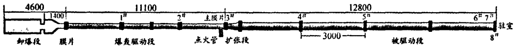
图7 长试验时间爆轰驱动实验装置结构示意图 Fig.7 Sketch of the experimental facility operated in a backward detonation expansion mode for long test time
