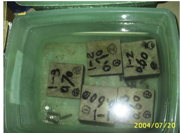
Fig. 1. Samples immersed in sodium sulfate solution for rebound test.
