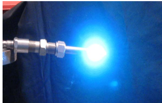
Figure 2. Discharging of the 50 J/pulse spark plug.
