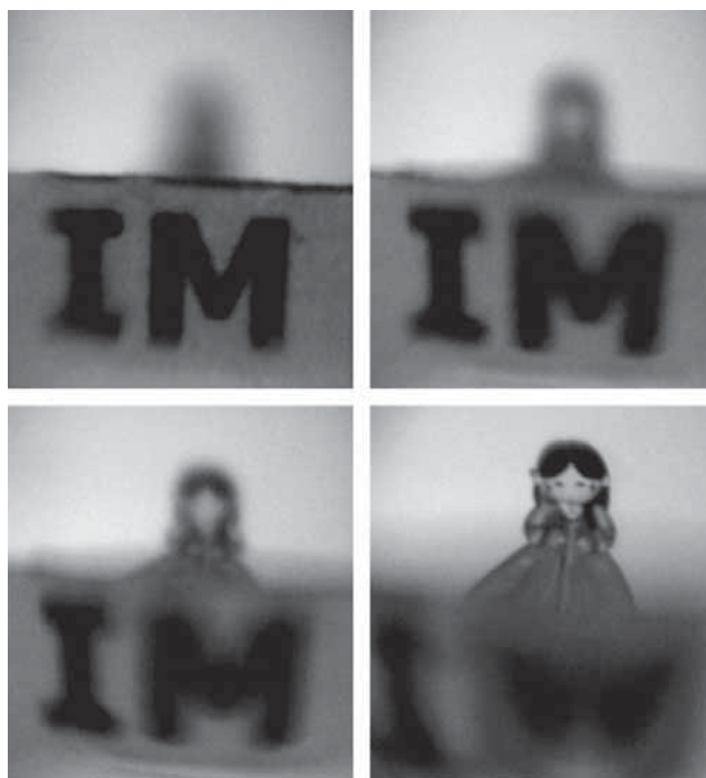
Figure 25 Images showing the ability of the EW based fluid lens. The focal plane is moved due to the EW effect. The letters 'IM' are placed closer to the lens than the doll. When the applied voltage is changed, the focal plane is moved from near to far, so the letters 'IM' and the doll are sequentially focalized [169].
