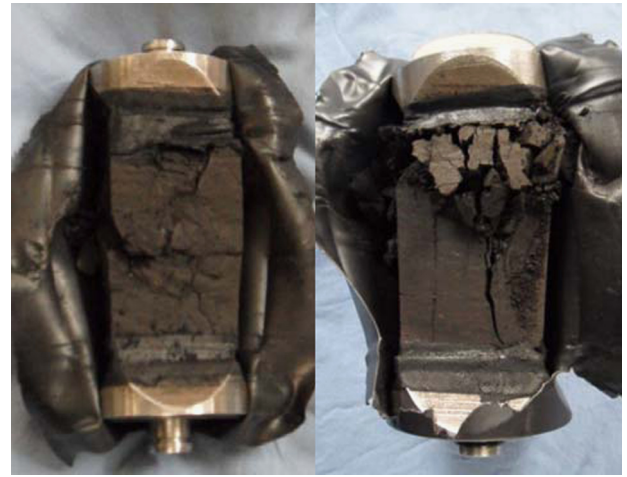
Fig. 7. The destruction of coal sample.
