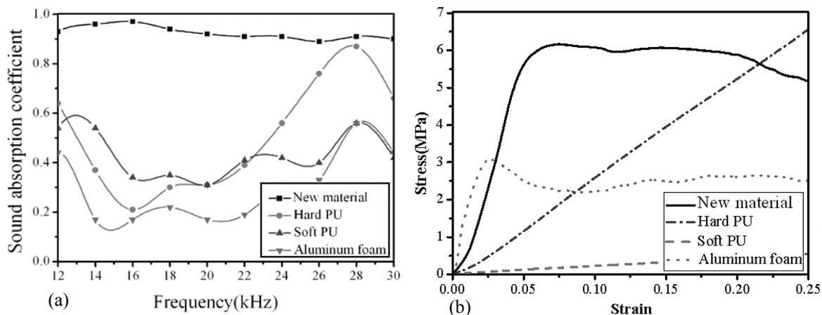
Fig. 1 - (a) Underwater absorption coefficients for different materials; (b) Compressive stress-strain curves of the new material and its component materials.
