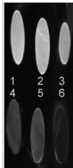
Figure 3. Ellipsometric image of air-stable chitosan-cushioned PEGylated lipid membrane. The numbers indicate different molar ratios of DSPE-PEG 2000 , which are 0.1, 0.25, 0.5, 1.5, 2.5, and 5 mol %, respectively.
