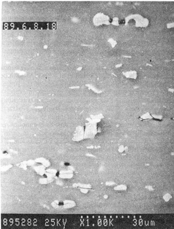
Fig. 3 Microcracks formed in specimen under short stress pulse loading
