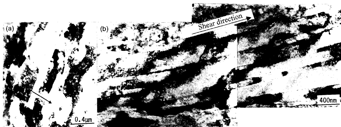
Fig.10 Recrystallization grains (a) and elongated cell structure (b) in the shear band produced during dynamic compression in Al/SiC p composite
