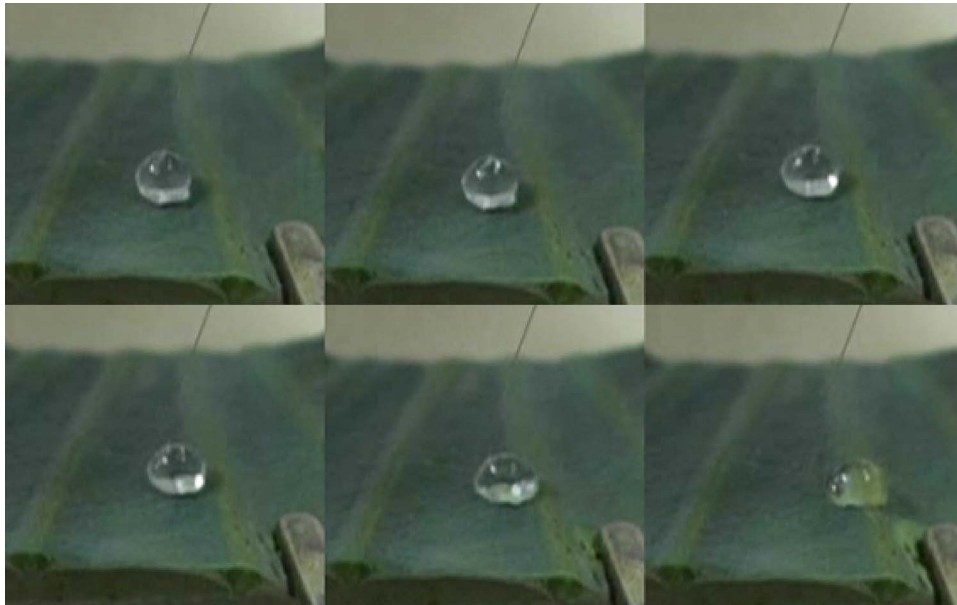
FIG. 4. Video sequence of the moving droplet induced by voltage. The whole process was caught by a Sony camera. The interval of each picture is 200 ms.
