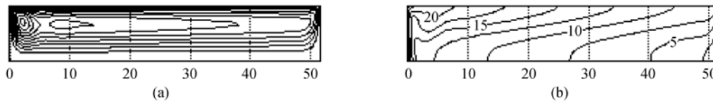
Figure 10 Average stream function (left) and isotherms in the liquid layer (right). g = 0, \Delta T = 25^\circ\text{C} .
