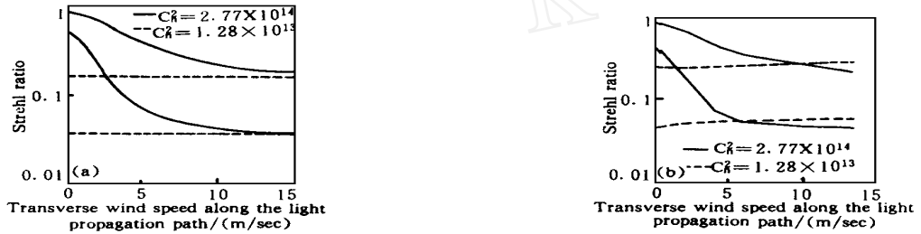
Fig 5 Relationship between Strehl ratio of the 37-element adaptive optics system and transverse wind speed along the light propagation path about spherical wave. The dashed lines are corresponding to the open-loop condition. (a). obtained from theoretical analysis, (b). obtained from numerical simulation
