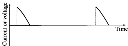
Fig. 9 Schematic drawing of pulse current
